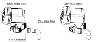
\*Control valve should be higher than sewer. The length of drain line should be similar to the height of tank. Insert the drain line to the floor drain, but not to the bottom. Leave about 15~25mm distance between the end port of drain line and sewer.
