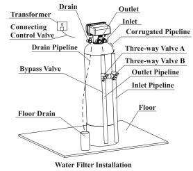
Illustration:Install three ball valves to connect the control valve and inlet/outlet pipeline. The valve B is connected with the inlet of the control valve; The valve A is connected with the outlet of the control valve. When repair the tank, adjust the valve A and B to make the inlet connected with outlet directly, so the water do not pass through the valve; When normally use, adjust the vale A and B connected with valve.
