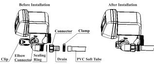
2.Use PVC hard tube for installation
